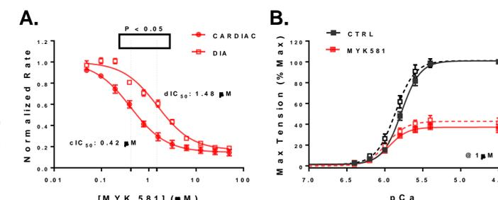
**Figure 2.** LEFT: DMSO normalized steady-state ATPase rates in cardiac (closed circles) and diaphragmatic (open squares) rat myofibrils exposed to MYK-581. RIGHT: Effect of MYK-581 (at 1 μM) treatment in tension-pCa curves at short (closed) and long (open) SL.
